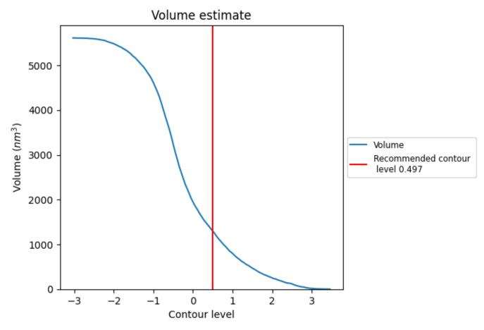
The volume at the recommended contour level is  $1300 \text{ nm}^3$ ; this corresponds to an approximate mass of 1175 kDa.
