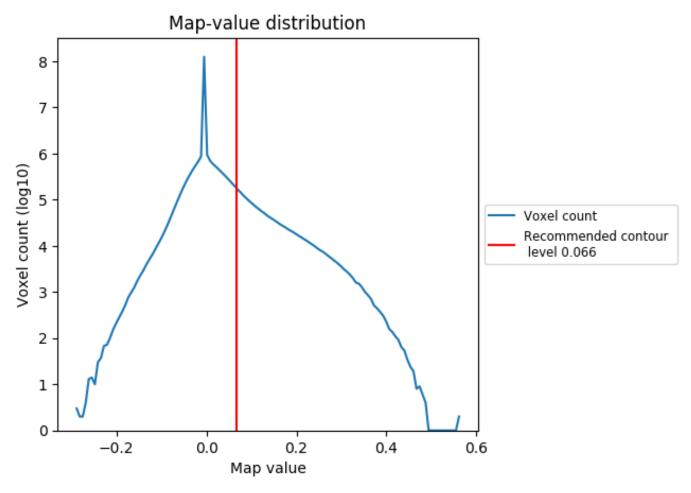
The map-value distribution is plotted in 128 intervals along the x-axis. The y-axis is logarithmic. A spike in this graph at zero usually indicates that the volume has been masked.
