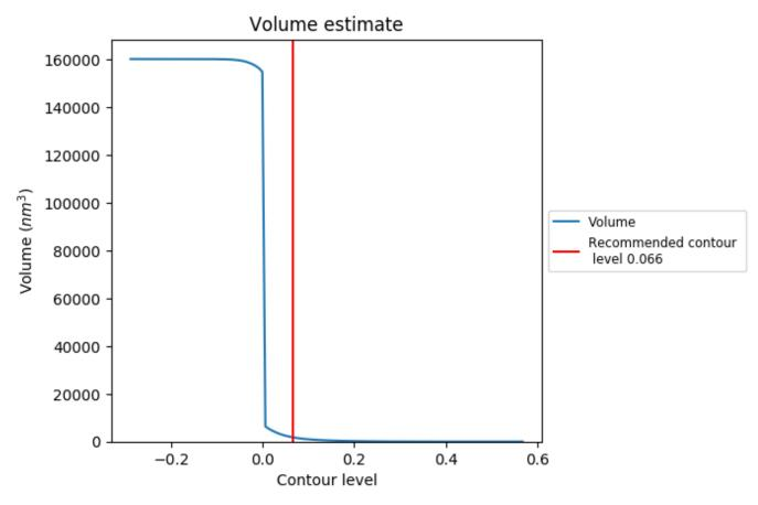
The volume at the recommended contour level is  $1776 \text{ nm}^3$ ; this corresponds to an approximate mass of 1605 kDa.
